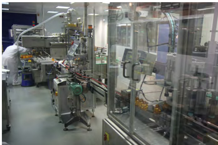
Pharmaceutical packaging line which produces authentic drug packaging for distribution.
